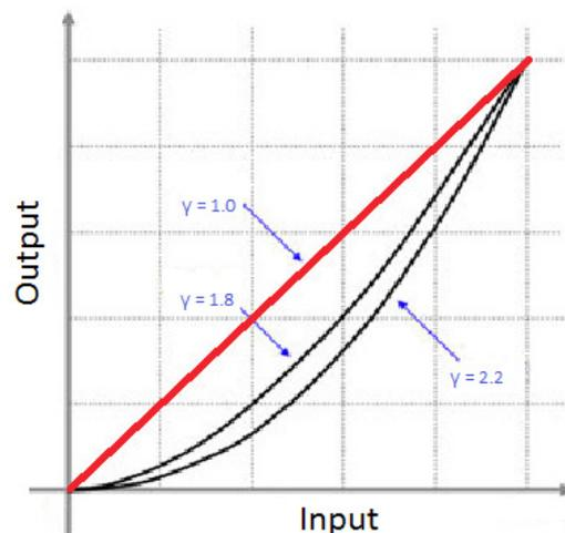
As the color reproduction of a display monitor is generally based on a combination of three primary colors: red (R), green (G), and blue (B), to obtain consistent color reproduction from light to dark shades, individual gamma correction for red, green, and blue channels is needed.
