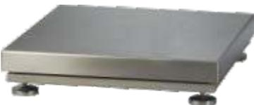
It consists of weighing pan (top cover) to keep load (material) and mechanical frames to transfer weight to loadcell. It will also have four adjustable feet for easy leveling and protection for loadcell from overload. Material of construction of top cover / frame, gauge of sheet / HSS used, painting & structural stability. These affect life and reliability of the scale.
