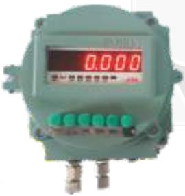
Enclosure, Zener barrier and loadcell approved by CMRI / ERTL / CCE for specific Zone and Group are used. If ignition occurs inside the enclosure, the enclosure will withstand the pressure and contain the internal explosion. The equipment becomes heavy and in few industries like pharma / food has to be enclosed by stainless steel cabinet for easy cleaning.
